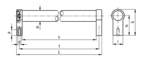
$\begin{array}{l} d &= M8 \\ d1 = 30 \\ f &= 300 \\ h &= 68 \\ h1 = 51 \\ L &= 317 \\ l1 &= 283 \\ p &= 15 \end{array}$
